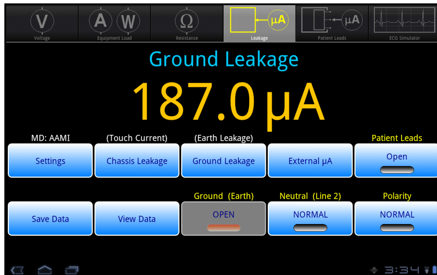
Figure 39 - Ground leakage display.
